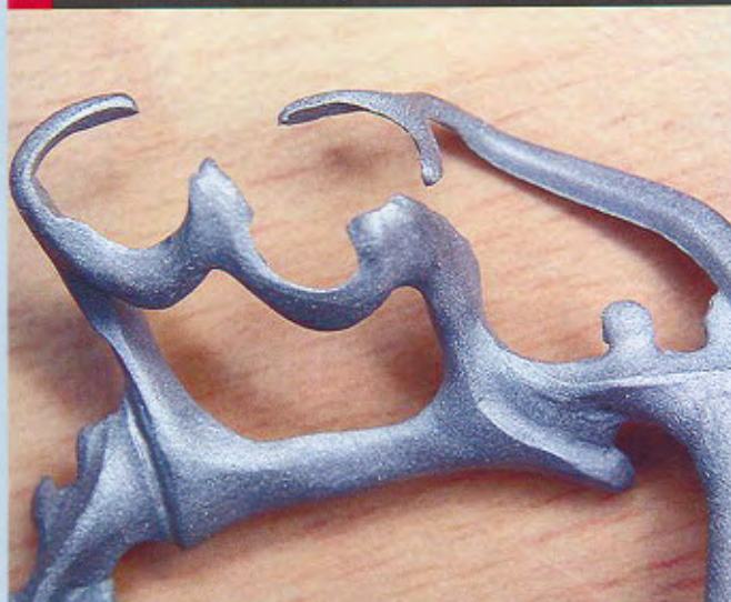
16 Framework after sandblasting: now just cut the sprues and polish.
